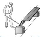
Let the lever come up and the lip will automatically extend to the positioned vehicle.
